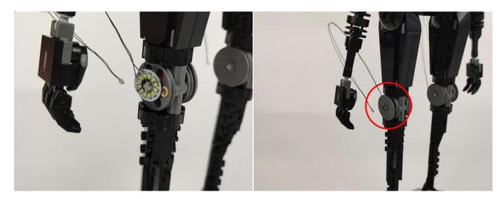
27. Twist the light wires of both arms and both legs into two strands.
