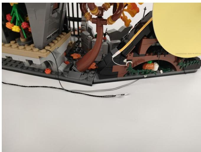
**65. Take out the 6 Socket Side-Mounted Expansion Board from "No. 3 bag". Twist the two black light wires on the left into a single strand and connect them to the expansion board. Connect the two light wires on the right to the expansion board separately.**
