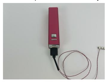
When we test the "①" lighting fixture, connect it to the expansion board, turn on the portable power bank, and the lighting fixture will light up normally, as shown in the figure below.
