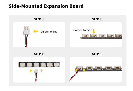
The connection method between the touch dimming module and expansion boards is as follows:
