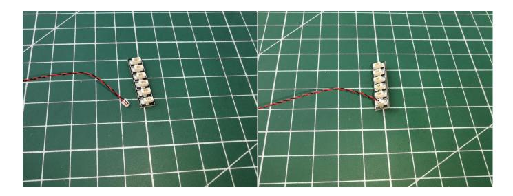
when we test "Bit Lights-15CM-Warm White" particles, Take out the bag labelled "Bit Lights-15CM-Warm White". Take out one of the light and connect it to the socket. Turn on the power bank, the light will turn on normally as shown below.
