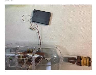
Take 2 adhesive squares and stick them on both ends of the 6-port expansion board. According to the slack of the cable, wrap the cable properly on the board, connect the plug to the board.
