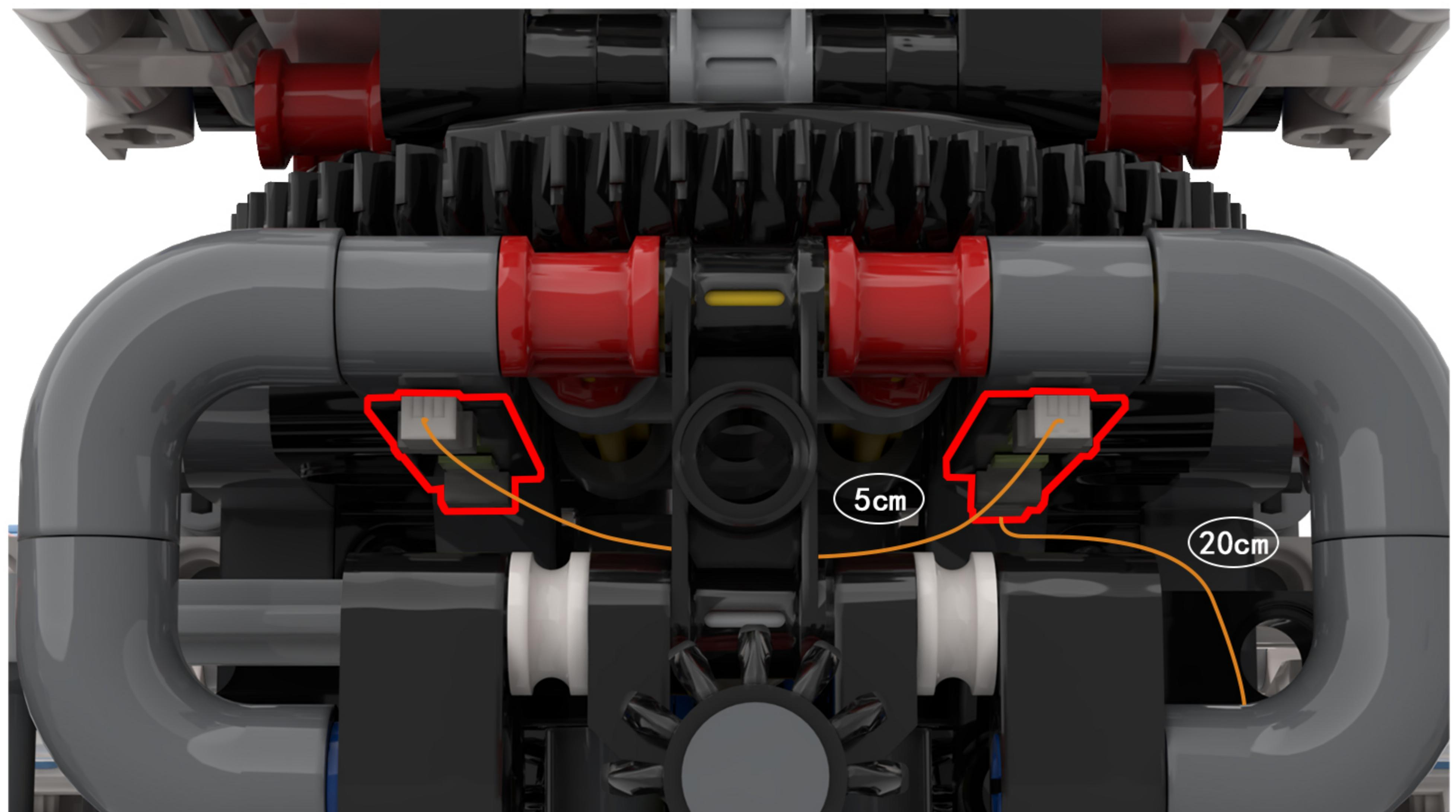
**Note:** Do not mix up the positions of the two light strips.
