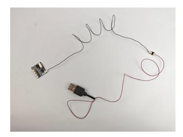
125.Connect the connecting wires to the corresponding ports on the module in order, then insert them into the interior of the building block, and finally restore the building block components.
