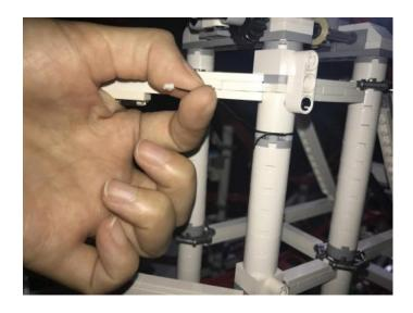
66.Take 3 warm white strips and 3 white 1x6 base plates, 2 connecting 5cm cables and a 50cm cable. Stick every strip on a plate, then, connect 3 cables to each of them.
