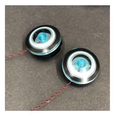
19.Reconnect the back wheels to the vehicle (ensuring the cables are at the lowest point of each wheel) and then from underneath, grab both cables and twist them around each other a few times.
