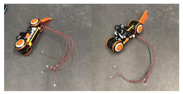
**57.Ensure cables are laid and facing the right side of the vehicle**
