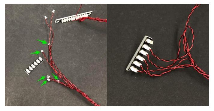
60.Connect the two longer cables from the orange vehicle to the
