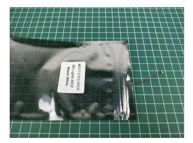
The components needs to be tested in this set is 2\*LED Strip Lights-Red,4\*LED Strip Lights-Blue,8\*LED Strip Lights-Warm White,13\*Bit Lights-30CM-Green,6\*Bit Lights-30CM-Warm White.
