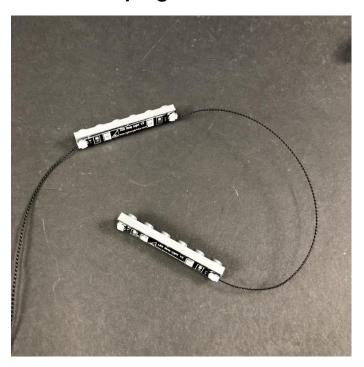
**125.**Connect the other end of the 15cm Connecting Cable from the Red Strip Light to the Blue Strip Light with a free port.
