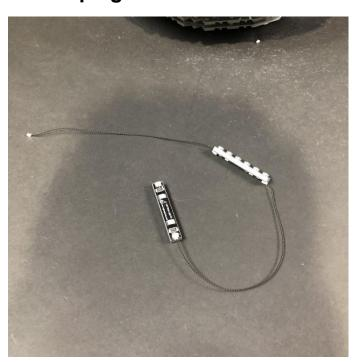
119. Take the other end of the 15cm connecting cable from the Blue Strip Light and connect it to the Red Strip Light that has a free port.
