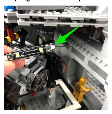
137. Mount the two White Strip Lights to the top of the Tie Fighter room in the below positions. Remember to loop excess cable in between strip lights underneath the 1x6 plate.
