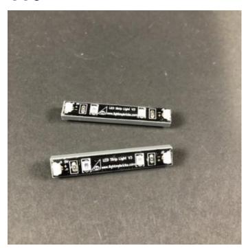
111. Take 2x 15cm Connecting Cables and connect one between the two strip lights and other other to the outside port of one of the strip lights.
