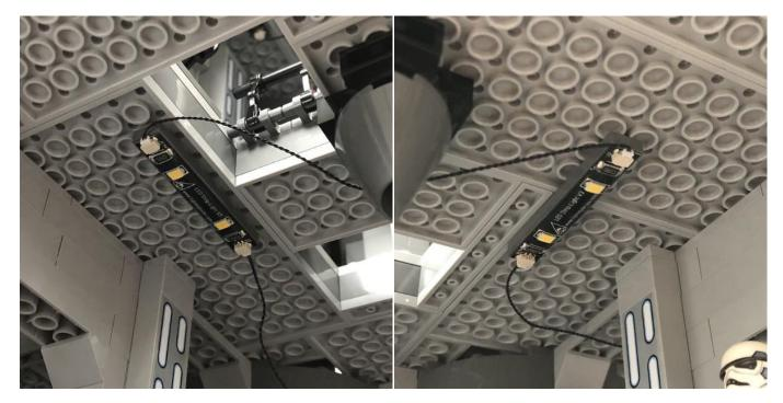
**194.**Thread the 30cm connecting cable down through hole on the left which leads the bottom space where the 50cm connecting cable from step 34 is.
