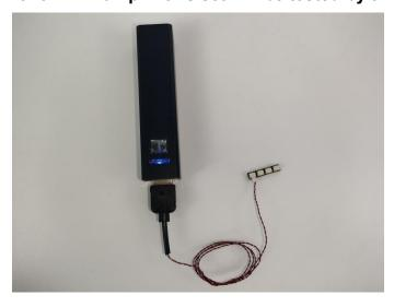
When we test the "2" lighting fixtures, remove one of them and connect it to the socket. Turn on the portable power bank, and the light strip will light up normally, as shown in the figure below.
