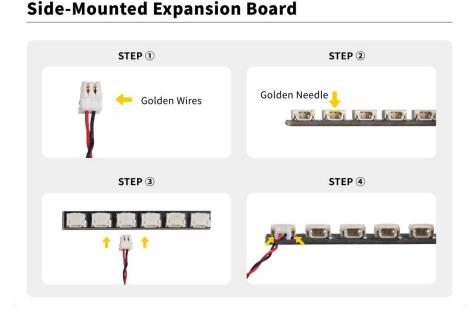
All our connections between plug and socket are all the same as shown above. So for any such structure with plug and socket, please pay attention to the golden wire of the plug and
