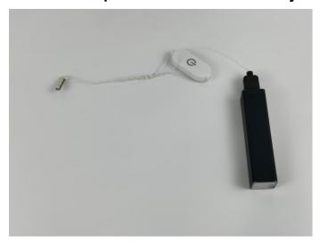
When we test the "①" lighting fixtures, remove one of them and connect it to the socket. Turn on the portable power bank, and the light strip will light up normally, as shown in the figure below.
