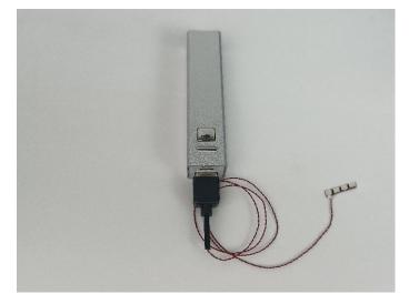
When we test the "④" lighting fixtures, remove one of them and connect it to the socket. Turn on the portable power bank, and the light strip will light up normally, as shown in the figure below.
