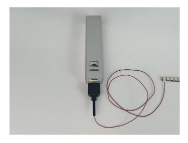
When we test the "④" lighting fixtures, remove one of them and connect it to the socket. Turn on the portable power bank, and the light strip will light up normally, as shown in the figure below.
