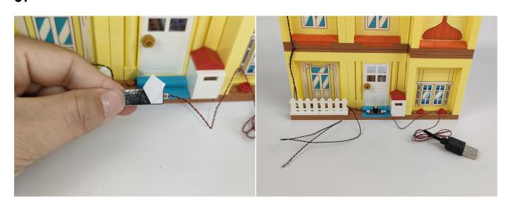
38.Press the connecting wires and power cord on the expansion board onto the bottom of the model, pull them to the side, and finally, flip the model over to the back. Then, temporarily place it aside.
