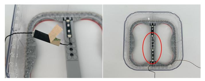
17.Gently tear off the light strip, place the wire and the light strip wire together, and then press the light strip back tightly against the glass wall.
