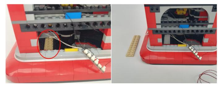
50. Thread the power cord from the inside of the base to the outside.
