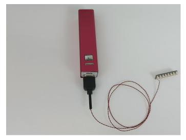
When we test the "①" lighting fixture, connect it to the expansion board, turn on the portable power bank, and the lighting fixture will light up normally, as shown in the figure below.
