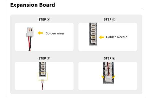
The connection method between the usb power cable and expansion boards is as follows:
