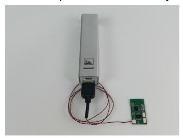
When we test the "①" lighting fixtures, remove one of them and connect it to the colorful remote control version. Turn on the portable power bank, and the light strip will light up normally, as shown in the figure below.
