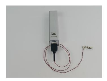
When we test "①" particles. Take out one of the light and connect it to the socket. Turn on the power bank, the light will turn on normally as shown below.
