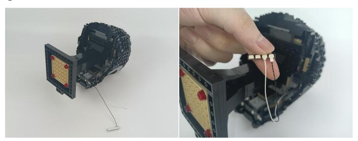
$\mathbf{9}_{ t t}$  Connect the cable to the "OUT" port on the light control module.
