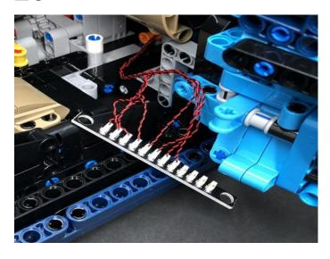
Take the AA Battery Pack and insert 3x AA Batteries to it. Connect the battery pack cable to the expansion board and then turn it ON to verify all lights are working OK.
