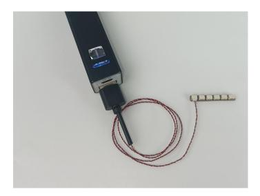
When we test "A01007 Light-30CM Yellow" particles, Take out the bag labelled "A01007 Light-30CM Yellow". Take out one of the light and connect it to the socket. Turn on the power bank, the light will turn on normally as shown below.
