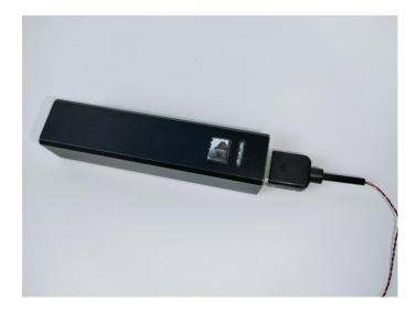
When we test "A02551 Light Strip-Warm White-COB" particles, Take out the bag labelled "A02551 Light Strip-Warm White-COB". Take out one of the light and connect it to the socket. Turn on the power bank, the light will turn on normally as shown below.
