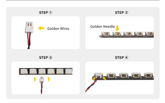
All our connections between plug and socket are all the same as shown above. So for any such structure with plug and socket, please pay attention to the golden wire of the plug and the golden needle of the socket, they must be touched together.
