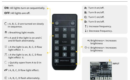
The remote control does not contain batteries, please buy a CR2025 or CR2032 button battery in the nearest store and install it in the remote control.
