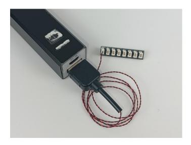
When we test "A01023 High-Brightness Light 30CM-Warm White" particles, Take out the bag labelled "A01023 High-Brightness Light 30CM-Warm White". Take out one of the light and connect it to the socket. Turn on the power bank, the light will turn on normally as shown below.
