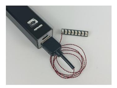
When we test "A1035 High-Brightness Light 15CM-Blue" particles, Take out the bag labelled "A1035 High-Brightness Light 15CM-Blue". Take out one of the light and connect it to the socket. Turn on the power bank, the light will turn on normally as shown below.
