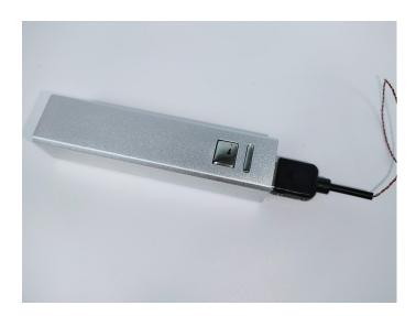
When we test "A1032 High-Brightness Light 30CM-Red" particles, Take out the bag labelled "A1032 High-Brightness Light 30CM-Red". Take out one of the light and connect it to the socket. Turn on the power bank, the light will turn on normally as shown below.
