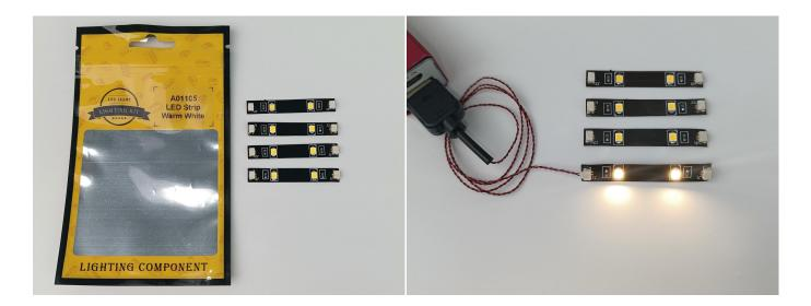
The components needs to be tested in this set is 2\* Disc shaped light - White-15cm,1\* Light Strip-Red,4\* Light Strip-Warm White-COB,4\*High-Brightness Light 15CM-Red.
