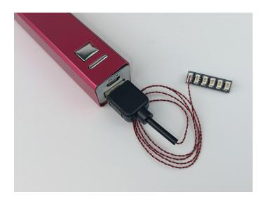
When we test "A01014 Light-15CM Orange" particles, Take out the bag labelled "A01014 Light-15CM Orange". Take out one of the light and connect it to the socket. Turn on the power bank, the light will turn on normally as shown below.
