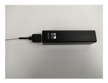
When we test "A1037 High-Brightness Light 15CM-Cyan" particles, Take out the bag labelled "A1037 High-Brightness Light 15CM-Cyan". Take out one of the light and connect it to the socket. Turn on the power bank, the light will turn on normally as shown below.
