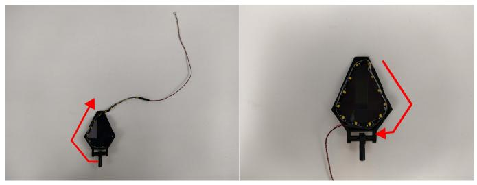
**5.**Thread the light wire through the block hole.
