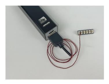
When we test "A01008 Light-30CM Blue" particles, Take out the bag labelled "A01008 Light-30CM Blue". Take out one of the light and connect it to the socket. Turn on the power bank, the light will turn on normally as shown below.
