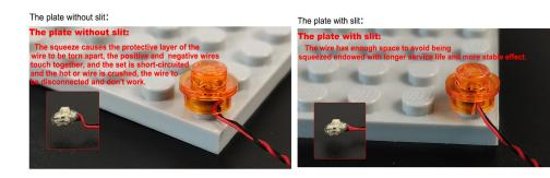
The slit on the plate round 1X1 are hand-made to avoid squeeze the wire and cause short circuit and abnormalheat during installation.
