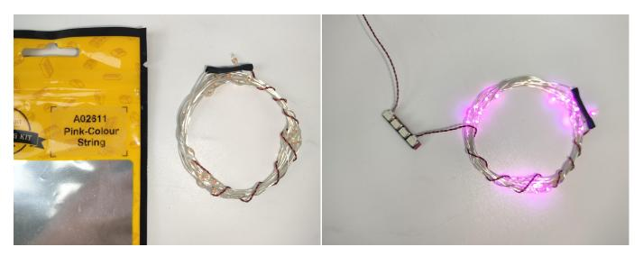
Test each lamp according to this method. It should be noted that after the test, the lamp must be returned to the corresponding bag to avoid confusion of types.
