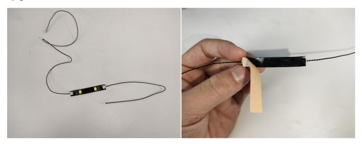
Attach the light strips to the block pieces, noting that the short side of the light wire is placed on the right side.
