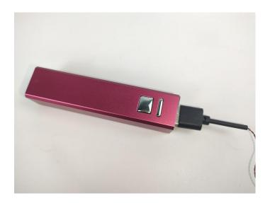
When we test "A01003 Light-15CM Red" particles, Take out the bag labelled "AA01003 Light-15CM Red". Take out one of the light and connect it to the socket. Turn on the power bank, the light will turn on normally as shown below.
