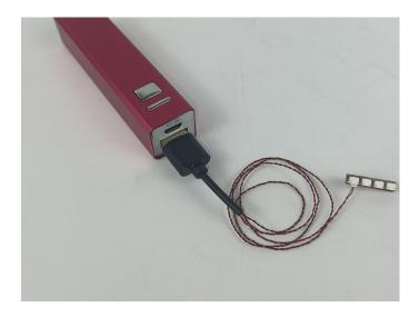
When we test "A02536 Light Strip-Warm White" particles, Take out the bag labelled "A02536 Light Strip-Warm White". Take out one of the light and connect it to the socket. Turn on the power bank, the light will turn on normally as shown below.
