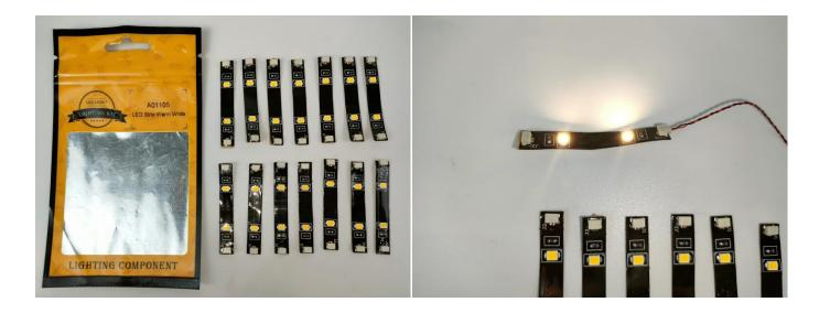
The components needs to be tested in this set is 3\* A01002 Light-15CM White,4\* A01003 Light-15CM Red,1\* A01024 High-Brightness light 15CM-Warm White,1\* A01025 Light-15CM Cyan ,1\*A02603 Warm White-Colour String.
