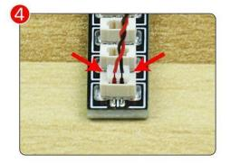
All our connections between plug and socket are all the same as shown above. So for any such structure with plug and socket, please pay attention to the golden wire of the plug and the golden needle of the socket, they must be touched together.
