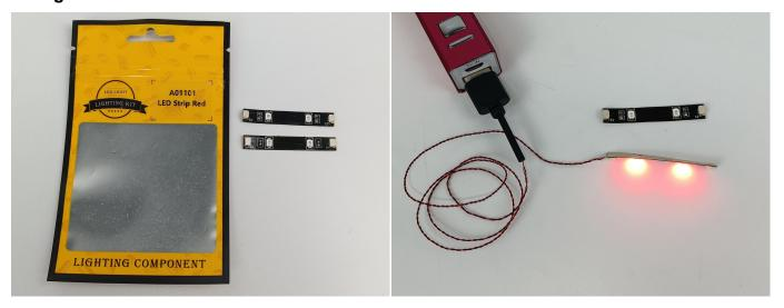
The components needs to be tested in this set is 2\* A1031 High-Brightness Light 15CM-Red, 2\*A1037 High-Brightness Light 15CM-Cyan.
