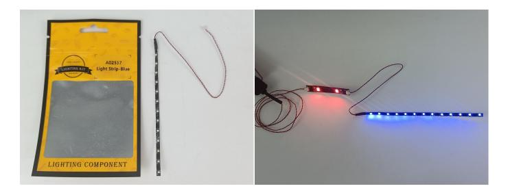
The components needs to be tested in this set is 2\* A01103 LED Strip Blue,1\*A01105 LED Strip Warm White.
