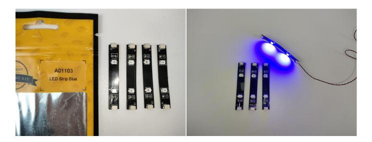
The components needs to be tested in this set is 2\* Light Strip-Blue,4\*Light Strip-Blue-COB.
