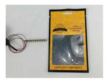
The components needs to be tested in this set is 3\*High-Brightness Light 30CM-Warm White,1\* Light Strip-Cyan-COB,1\* High-Brightness Light 15CM-White,2\* High-Brightness Light 15CM-Blue.
