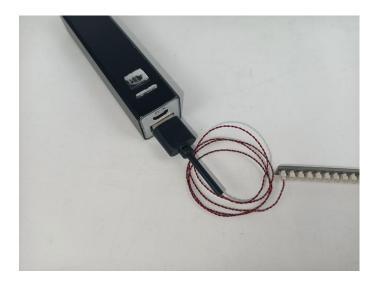
When we test "A1033 High-Brightness Light 15CM-Green" particles, Take out the bag labelled "A1033 High-Brightness Light 15CM-Green". Take out one of the light and connect it to the socket. Turn on the power bank, the light will turn on normally as shown below.
