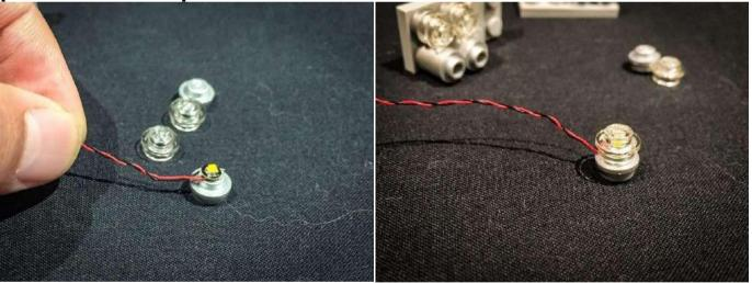
9.Install the remaining LEDs to all front headlights (2 on each side) using the above process so that we have a total of 4 standard Dot Lights installed. Reconnect the light pieces back to the 2 2x4 plates ensuring that the cables from the LEDs are facing upward and then reconnect the plates back to the front of the car.
