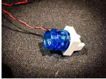
21.Reconnect this section back to the side of the car ensuring the cable from the LED is on the inside facing the car.
