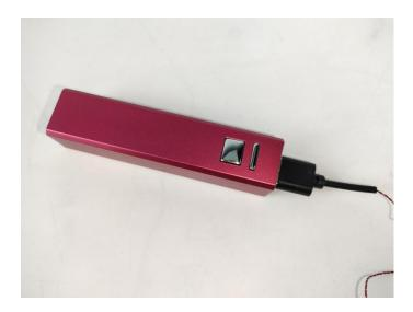
when we test "A1031 High-Brightness Light 15CM-Red" particles, Take out the bag labelled "A1031 High-Brightness Light 15CM-Red". Take out one of the light and connect it to the socket. Turn on the power bank, the light will turn on normally as shown below.
