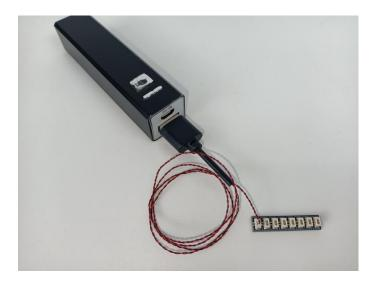
When we test "A02510 Light Strip-Cyan" particles, Take out the bag labelled "A02510 Light Strip-Cyan". Take out one of the light and connect it to the socket. Turn on the power bank, the light will turn on normally as shown below.
