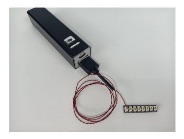
When we test "A01002 Light-15CM White" particles, Take out the bag labelled "A01002 Light-15CM White". Take out one of the light and connect it to the socket. Turn on the power bank, the light will turn on normally as shown below.
