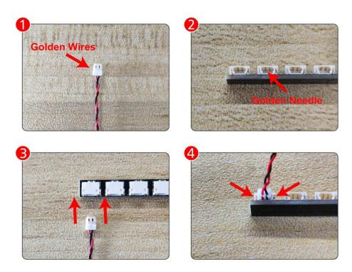
All our connections between plug and socket are all the same as shown above. So for any such structure with plug and socket, please pay attention to the golden wire of the plug and the golden needle of the socket, they must be touched together.
