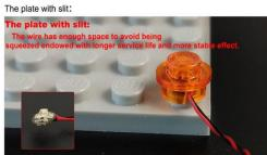
The slit on the the plate round 1X1 are hand-made to avoid squeeze the wire and cause short circuit and abnormalheat during installation.
