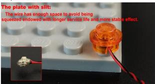
The slit on the plate round 1X1 are hand-made to avoid squeeze the wire and cause short circuit and abnormalheat during installation.
