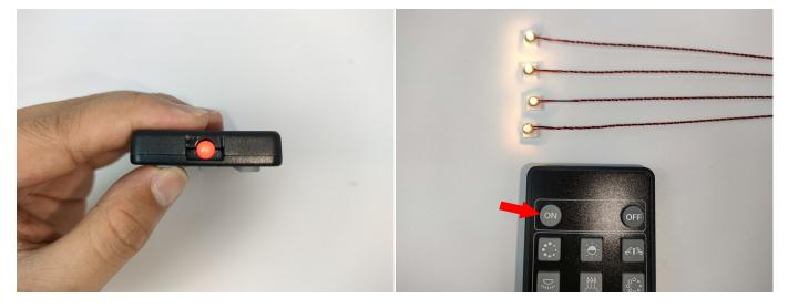
If there is any problem with the spare parts, please contact our after-sales service for replacement! When we test "A1029 High-Brightness Light 15CM-White" particles, Take out the bag labelled "A1029 High-Brightness Light 15CM-White". Take out one of the light and connect it to the socket. Turn on the power bank, the light will turn on normally as shown below.
