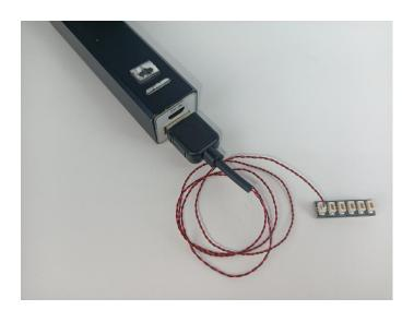
When we test "A01024 High-Brightness light 15CM-Warm White" particles, Take out the bag labelled "A01024 High-Brightness light 15CM-Warm White". Take out one of the light and connect it to the socket. Turn on the power bank, the light will turn on normally as shown below.
