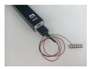
When we test "A01024 High-Brightness light 15CM-Warm White" particles, Take out the bag labelled "A01024 High-Brightness light 15CM-Warm White". Take out one of the light and connect it to the socket. Turn on the power bank, the light will turn on normally as shown below.
