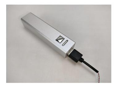
When we test "A02552 Light Strip-Blue-COB" particles, Take out the bag labelled "A02552 Light Strip-Blue-COB". Take out one of the light and connect it to the socket. Turn on the power bank, the light will turn on normally as shown below.
