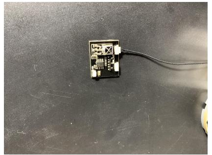
Connect the 15cm connecting cable from the lower floor to the input port (the smaller one) on the RGB board, secure the RGB board under the stairs by using the adhesive tapes. Then follow the next steps.
